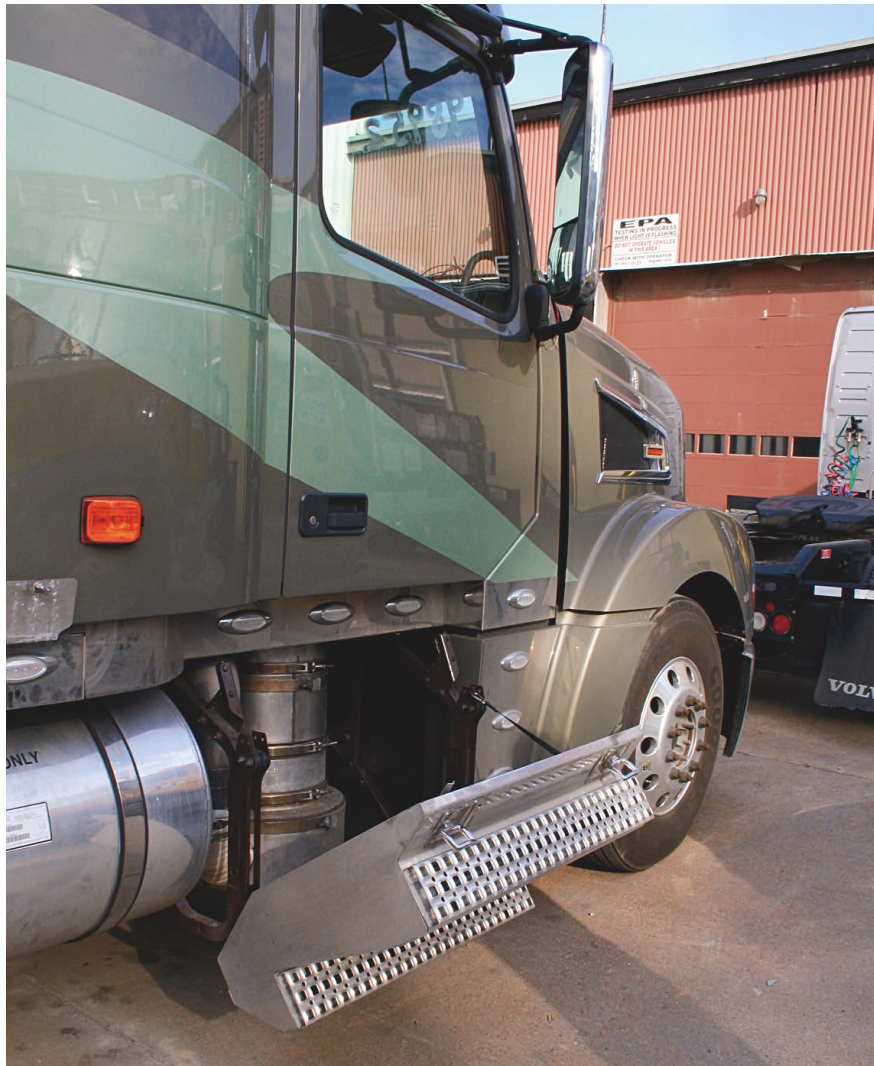
Certain Volvo and Mack truck models use a compact DPF that resides behind the right front wheel.
