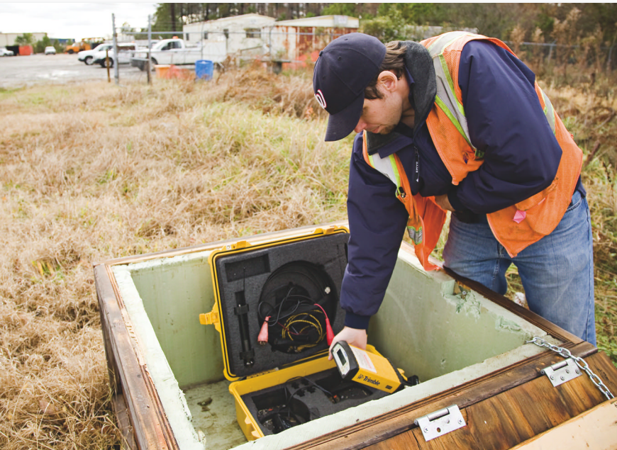
Above: Kyle Myers, project engineer and GPS manager for E.V. Williams Inc., looks over the Trimble SPS 880 base station housed inside a large wood crate.
