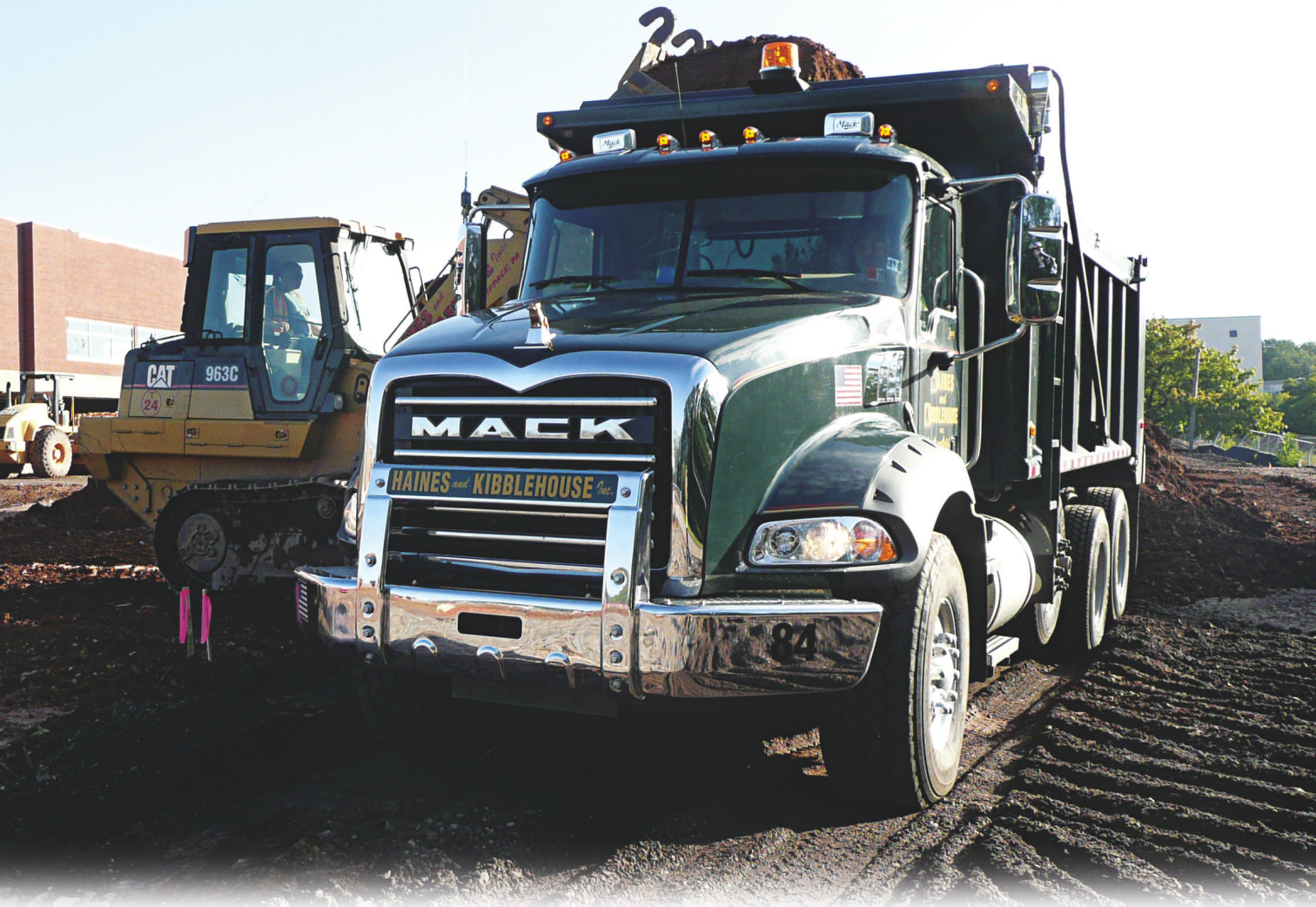
Green Granite with its 2010 SCR diesel is owned by Mack and was loaned to Haines & Kibblehouse for testing. It has worked well and fuel economy is encouraging.
