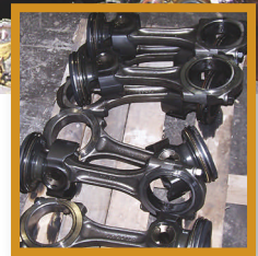
This 13,000-hour tear down of an engine from one of Fred Weber Corp.'s 988F wheel loaders shows the results of 7,000 hours running on Emissions Technology's diesel catalyst. Ed Moss, maintenance manager, says the evidence indicates the catalyst can extend engine life by about 5,000 hours. The catalyst cut the loader's fuel consumption by three gallons per hour.
