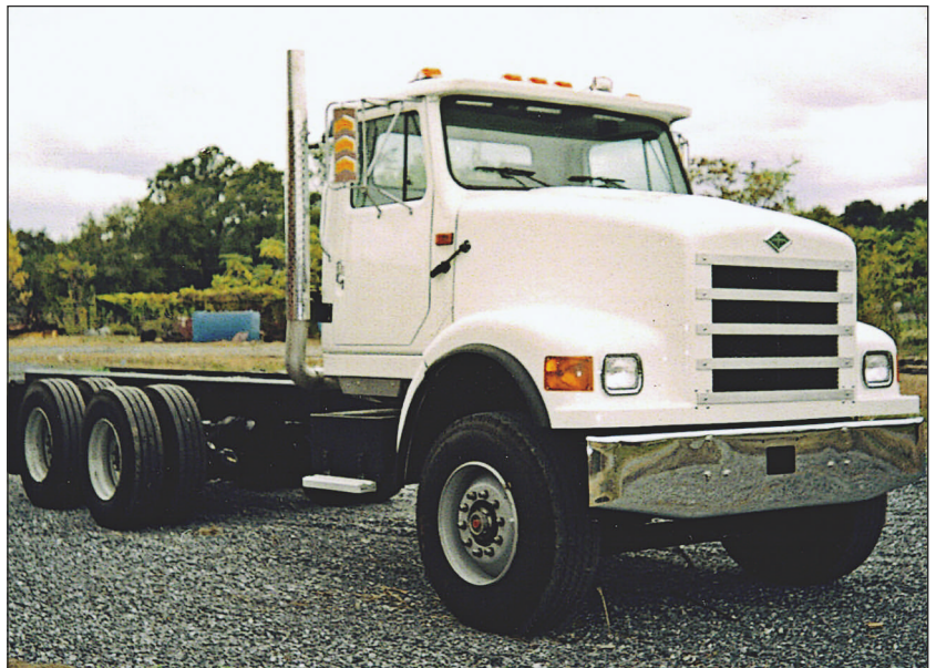
T-Line 5364V, one of three models from Diamond Vehicle Solutions in Harrisburg, Pa., is aimed at vocational users. It's standard with a Cat C7 diesel, Eaton manual transmission, and Dana axles. The cab is International's old S design, but a new cab is planned.
